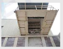
Some nonconforming wet plasters are dismissed from the system by the roll-out belt in the plasterboard production facility. This boards, being in from of mixed paper and gypsum powder with dimension of 5-15 cm are stored in the storage area, by being passed through the main shredder located on the outlets of roll-out belt.
